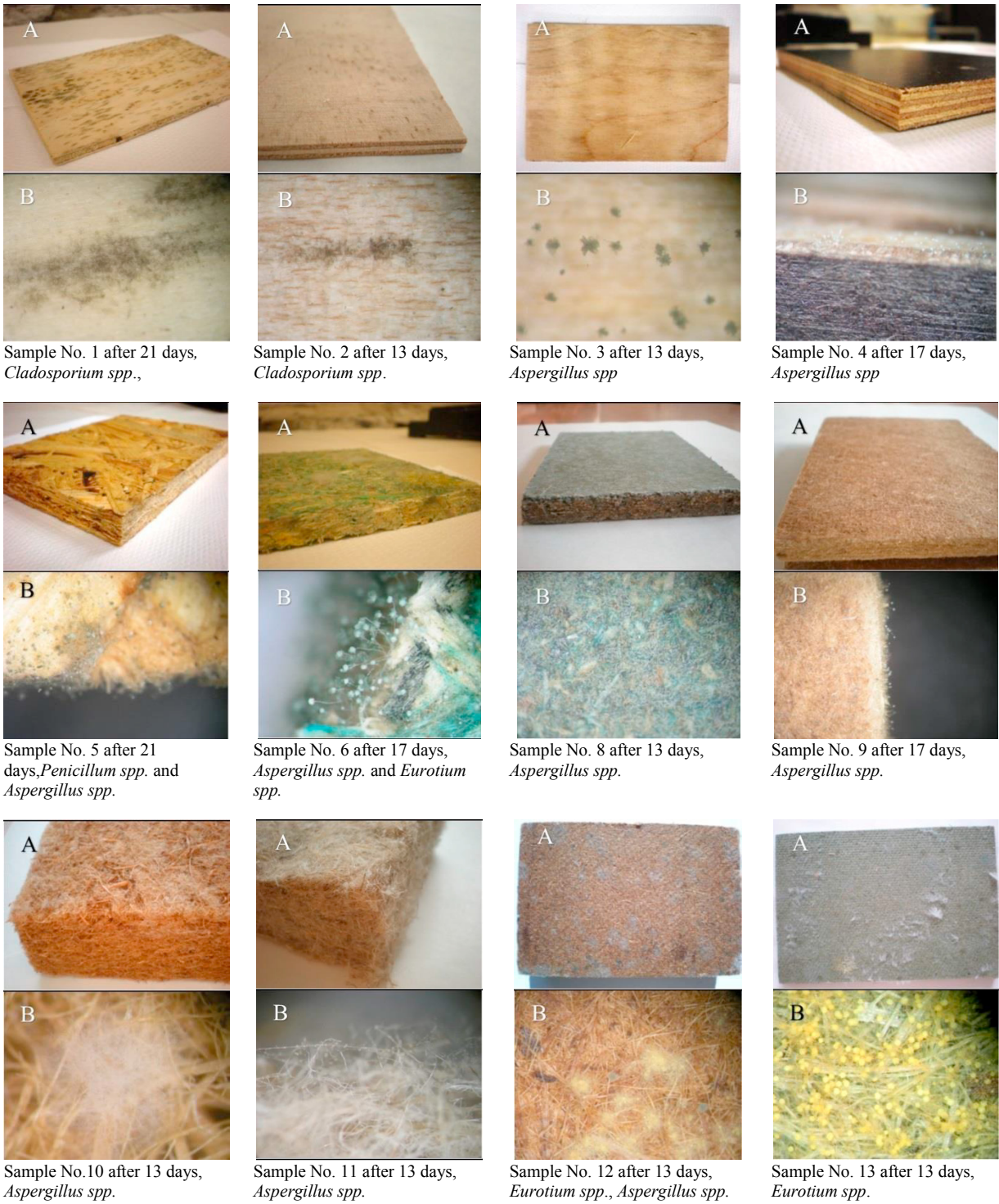
Fig. 2. Inspection of samples after the test: (A) visual inspection; (B) close-up view under the stereomicroscope.
